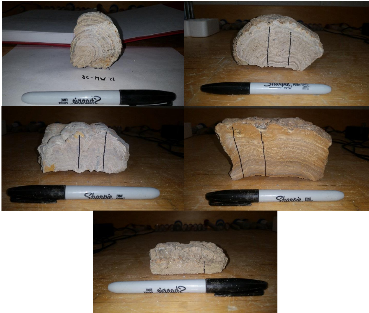
Figure 6. These images show the chosen sample stromatolites cut in half in order to determine the best area to sectionalize further and scan using XRCT. (Top Left: 15WM3, Middle Left: 15WM3A1, Top Right: 15WM4N, Middle Right: 15WM4G, Bottom: 15WM3Q)
