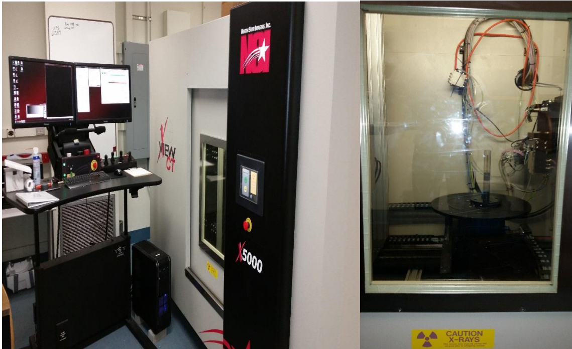
Figure 8. The left image shows the entire CT scanner along with the controlling computer system. The right image shows the inside of the machine as the calibration process is taking place before scanning begins.
