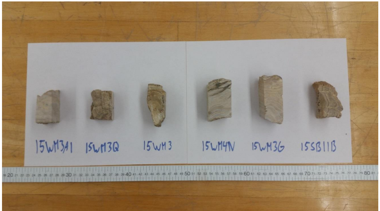
Figure 7. This picture shows the cuts made using a rock saw to trim the specimens into the proper sized samples, roughly 3cm by 5-7cm. (15SB11B was included to show diversity of stromatolites at various locations.)
