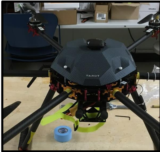
Figure 8- During the field research the GPS was located on the cover of the UAV, which can be seen in the image on the left. The new location of the GPS, image on the right, makes the inter-components of the UAV more accessible.
