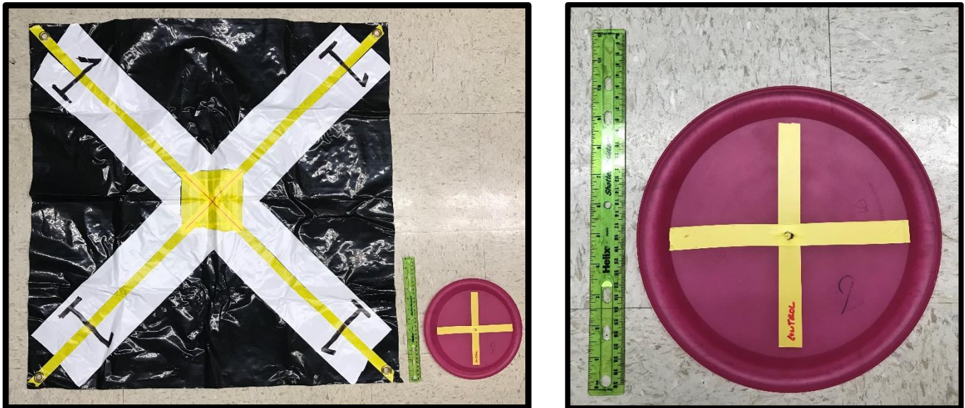
Figure 10- The new GCPs, seen in the left image being compared to the old GCPs, that will be used will be much more visible on the surface of the glacier as compared to the old GCPs seen in the image on the right.
