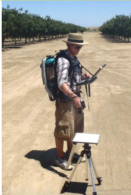
Brandon Furey ('12) measures ground reflectance using an $80,000 spectrometer backpack
