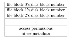
Figure 8.6: This initial approximation of an inode shows the principle categories of metadata. However, this diagram is unrealistic in that the list of disk block numbers seems to be unlimited, whereas actual inodes have only a limited amount of space.
