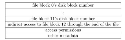
Figure 8.7: In this limited-size inode, blocks from number 12 to the end of the file are indirectly referenced.
