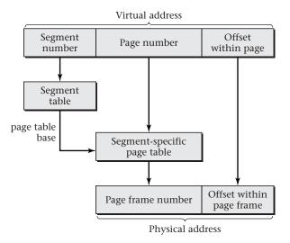
Figure 6.17: The Multics system combines segmentation and paging using a separate page table for each segment. The segment table is used to find the appropriate page table, which is then used to translate the address within the segment.
