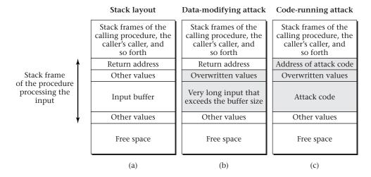
Figure 11.4: If input (shown in grey) is allowed to overflow the amount of memory allocated on the stack for an input buffer, it can overwrite other data values, as shown in part (b), or the return address, as shown in part (c). In the latter case, the modified return address can point to attack code included in the oversized input.
