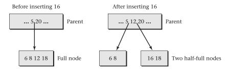
Figure 8.12: Inserting 16 into the illustrated B-tree, which has node-capacity 4, causes a node to split, with the median key moving into the parent.
