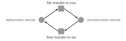
Figure 4.22: The cycle in this resource allocation graph indicates a deadlock. Each square represents a thread and each circle a mutex. An arrow from a square to a circle shows a thread waiting for a mutex, whereas an arrow from a circle to a square shows a mutex being held by a thread.
