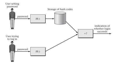
Figure 11.1: The system stores a cryptographic hash of the password when it is set, and compares that with the hash of the attempted password. Because the hash function is collision-resistant, equal hashes mean the password was almost surely correct. Because the hash function is difficult to invert, disclosure of the stored hash codes would not reveal the passwords.
