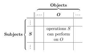
Figure 7.10: An access matrix has one row for each subject, one column for each object, and entries showing which operations each subject can perform on each object.
