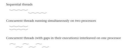
Figure 2.2: Sequential and concurrent threads
