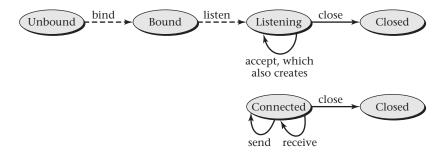
Figure 9.6: This state diagram shows the life cycle of server-side stream sockets used to accept TCP connections. In the Java API, the class <code>java.net.ServerSocket</code> is used for this purpose, and the bind and listen operations ordinarily are performed automatically as part of the constructor. Each time the accept operation succeeds, a new connected socket is returned, which in the Java API is an instance of <code>java.net.Socket</code>.
