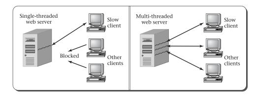
Figure 2.5: Single-threaded and multithreaded web servers
