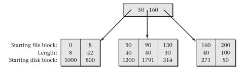
Figure 8.13: This small  $B^+$ -tree extent map contains information that can be used to find each extent's range of file block numbers and range of disk block numbers. Because the tree is a  $B^+$ -tree rather than a B-tree, all the extents are described in the leaves, with the nonleaf node containing just navigational information.
