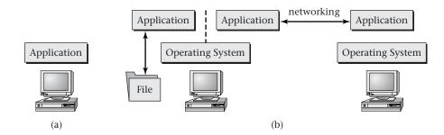
Figure 1.1: Without an operating system, a computer can directly execute a single program, as shown in part (a). Part (b) shows that with an operating system, the computer can support concurrent computations, control the interactions between them (suggested by the dashed line), and allow communication across time and space by way of files and networking.
