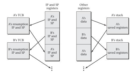
Figure 2.8: Saving registers in thread control blocks and per-thread stacks
