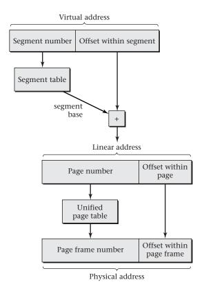
Figure 6.16: The IA-32 architecture combines segmentation and paging using a single page table for all the segments. The segment table is used to translate the segment number into a base address, to which the offset within the segment is added, yielding a linear address. The linear address is then translated to a physical address using the unified page table, as shown in greater detail in Figure 6.14.
