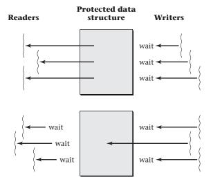
Figure 4.15: A readers/writers lock can be held either by any number of readers or by one writer. When the lock is held by readers, all the reader threads can read the protected data structure concurrently.
