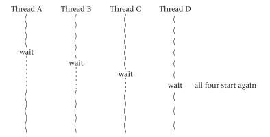
Figure 4.16: A barrier is created for a specific number of threads. In this case, there are four. When the last of those threads invokes the wait operation, all the waiting threads in the group start running again.
