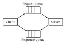
Figure 10.2: A client and server can engage in a request-response protocol using two message queues. Typically, the client tags each request message with a unique identifying string, known as a *correlation ID*. The server copies this ID into the resulting response message so that the client knows to which request the response corresponds.
