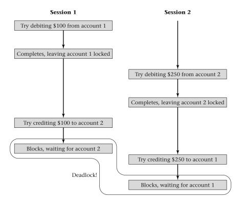
Figure 5.2: Two transfer transactions deadlock when each waits for exclusive access to the account for which the other already has obtained exclusive access. In this diagram, the vertical dimension represents the passage of time.
