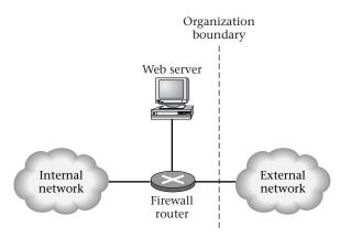
Configuration of the firewall router:
