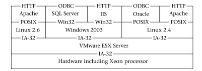
Figure 7.18: This example shows a VMM, the VMWare ESX Server, supporting multiple operating systems. The label within each box identifies a component, whereas the label on each horizontal dividing line identifies an interface. Unlike the operating systems, the VMM provides upward the same IA-32 interface that it relies upon from below.
